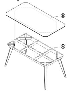
From beneath, secure the Table Top (B) to the Frame (A) using the Screws (G) provided as shown. Assembly is now complete.
