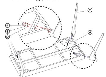
2 Carefully lift and rotate the table assembly rightside up. Place the Top (B) on top of the Frame (A).
